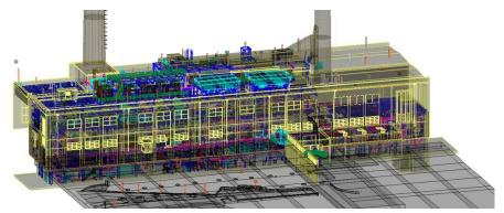
Due to the vast space and density of piping, it would have been difficult and time consuming to accurately depict the location of pipe runs, structural features and other details in the plant manually.
